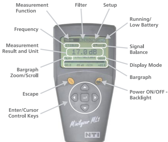
Fig 2.1 Display & Control Elements
