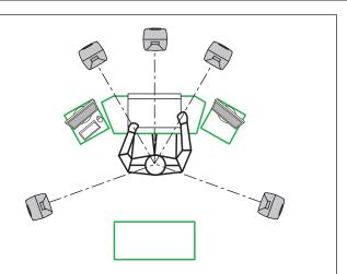
Figure 4. Symmetrical layout and keeping the acoustic axis clear from obstructions minimizes reflection surfaces and maintains accurate localisation because reflections are symmetrical.
