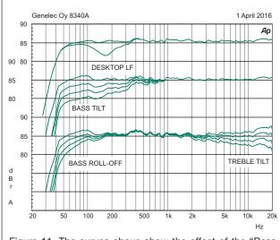
Figure 11. The curves above show the effect of the "Bass Tilt", "Treble Tilt", "Desktop Low Frequency" and "Bass Roll-Off" controls on the free field response of the 8340A.
