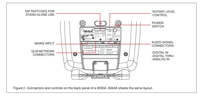
These monitors produce 100 dB SPL sound level at 1 meter in free space for a digital input signal of -30 dBFS. The DIGITAL OUT male XLR carries an unaltered copy of the digital signal fed into the digital in connector. This enables daisy-chaining up to four monitors.
