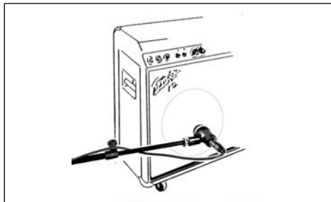
Fig. 3: Microphone placement for a guitar amp.
