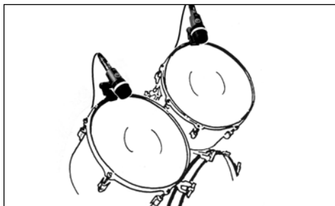
Fig. 5: Aligning the microphone with a tom-tom or roto tom.
